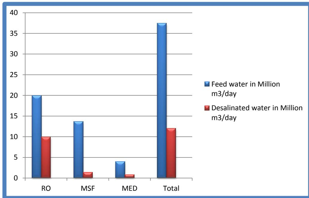
Figure 16: Estimated daily volume of feed water withdrawn from the Mediterranean compared to production of desalinated water using different desalination technologies in million m<sup>3</sup>/day during the year 2013.
