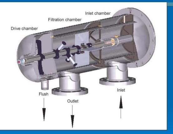
Source Water Enters Inner Side and Moves Radially Through the Screen
