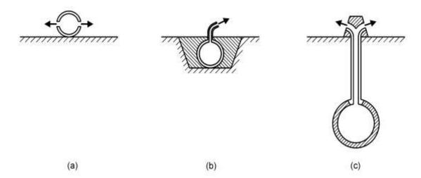
Figure 20: Typical construction details for multiport diffusers in water bodies: (a) Diffuser pipe on bottom with port holes, (b) diffuser pipe buried in trench with short risers, (c) deep tunnel construction with long risers
