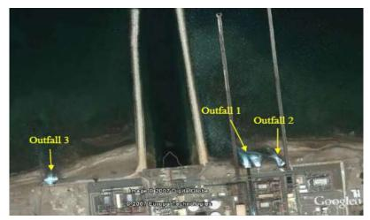
Figure 16: Al Gubrah (Oman), MSF plant, 191,000 m<sup>3</sup>/d, Gulf of Oman, positively buoyant discharge (Source: Google Earth)
