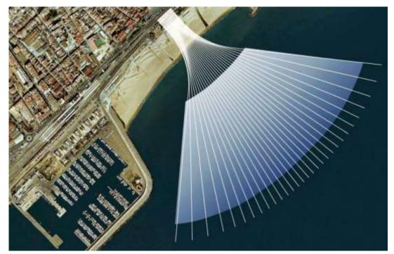
Figure 5: Several horizontal subseabed drills with filtration region shown in light blue (Neodren system, Peters and Pinto, 2006).
