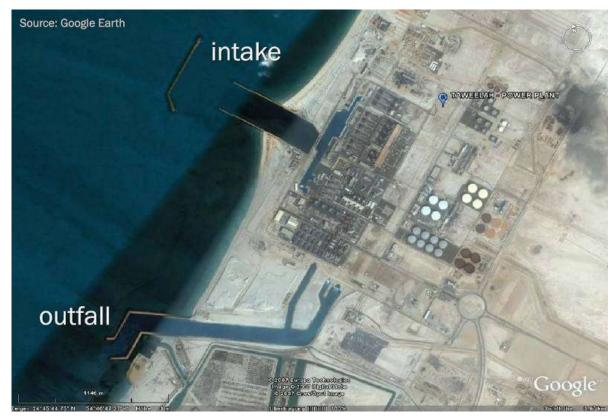
Figure 18: Taweelah MSF plant, Arabian Gulf, 1.12 mio m<sup>3</sup>/d, positively buoyant discharge (Source: Google Earth)
