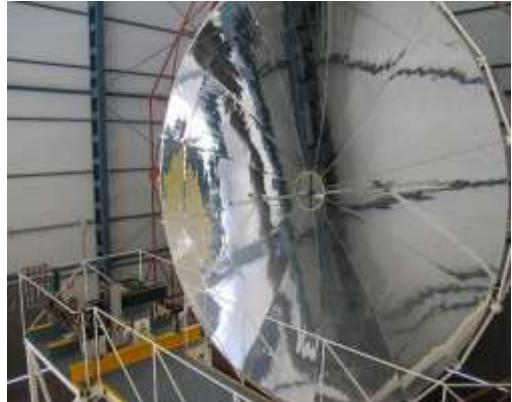
Fig. 15. Interior view of the SF-40 solar furnace, showing the parabolic concentrator
