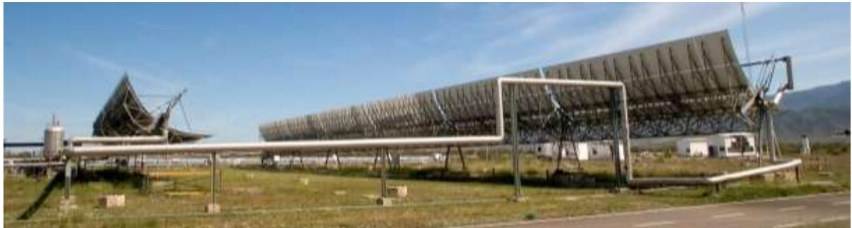
*Fig. 5. PSA "HTF test Loop"*
