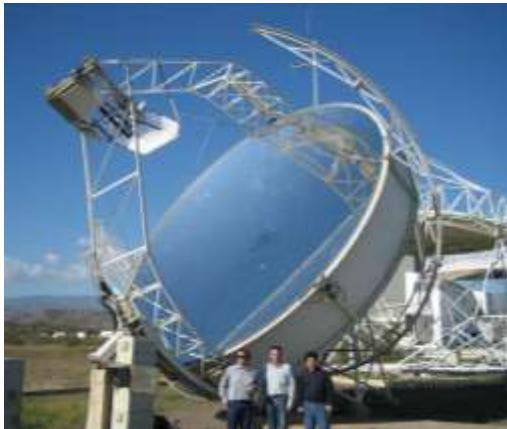
*Fig. 9. Parabolic-dish DISTAL-I used for accelerated materials ageing*
