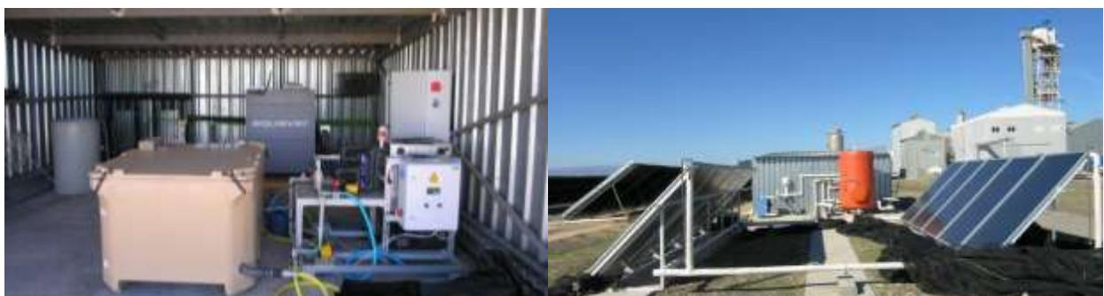
*Fig. 20. Internal (left) and external (right) views of the Membrane Distillation experimental test bed within the PSA low-temperature solar thermal desalination facility*
