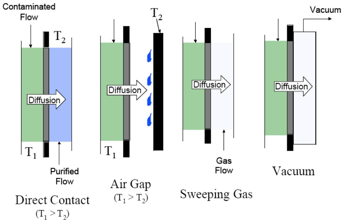
Figure 9: Different membrane distillation process
