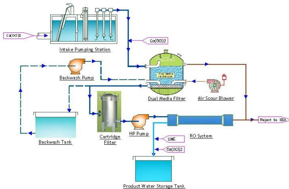
Figure 5: SWRO process schematics
