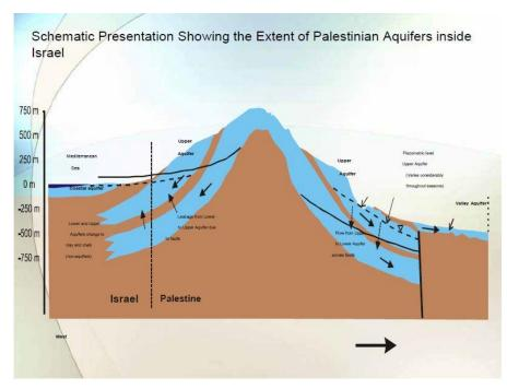
Figure 5. Hydrogeological cross-section West Bank (Amjad Aliewi, 2006)
