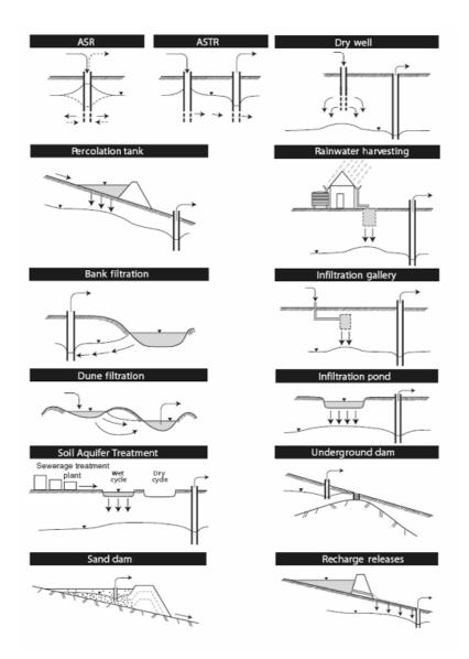
Figure 1. Systems for Managed Aquifer Recharge(see also text box)
