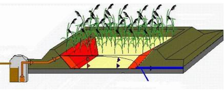
Horizontal subsurface flow (H-SSF)
