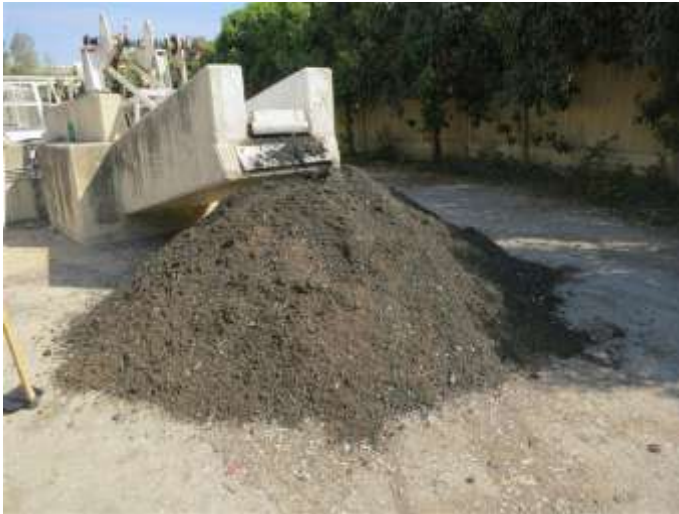
Figure 8 Grit discharged by classifier
